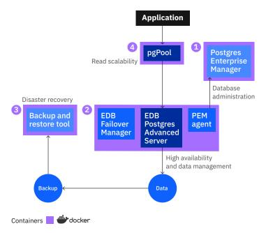
Figure 3. Recommended containerized deployment of EDB
