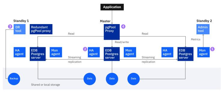
Figure 2. Standard (not containerized) high-availability Postgres database deployment
